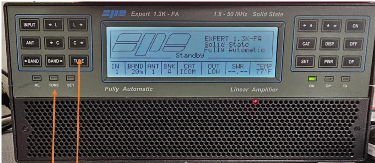
3. Press the TUNE Button on the amplifier (The TUNE LED illuminates) and immediately press the TRANSMIT button on the IC-7300.
