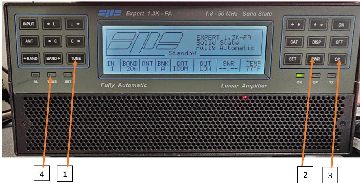
When the amplifier is first powered on it will be in the Stand-By mode. The amplifier can only be tuned in the Stand-By mode.
