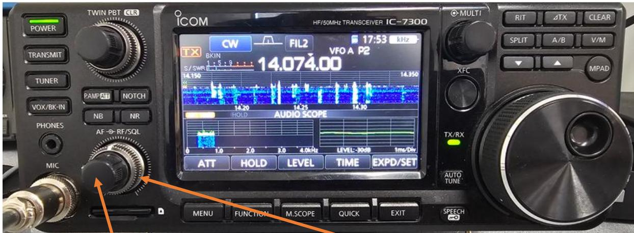
Volume Control (Center) - RF Gain Control (Concentric)
