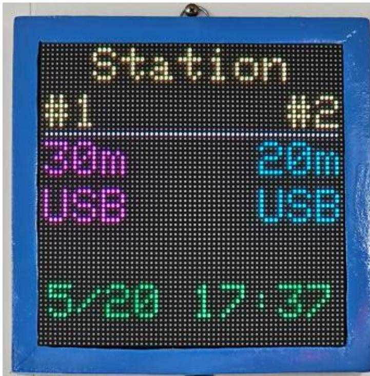
The station status monitor will initiate a warbling tone alert if both stations are set to the same band for more than 3 seconds. To disable the alert, change the band on either station #1 or station #2. If a station is set to a frequency that is out of band the band display will show “???”.
