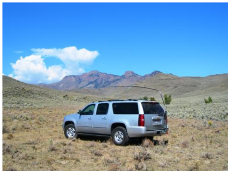
Suburban with Bent Over Whip for NVIS Communications
