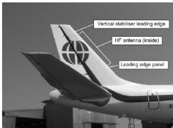
Large Jet with HF Antenna Located inside the Tail Fin for Automated Reporting and Comms
