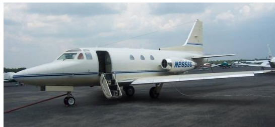
Sabreliner Jet with 23' Wire Antenna for Global HF ALE Comms
