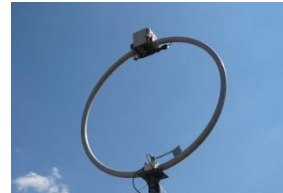
Loop Antenna (low freq noise reduction)
