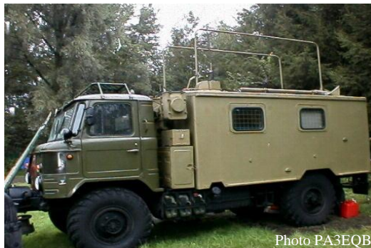
Russian Radio Vehicle with NVIS Antenna
